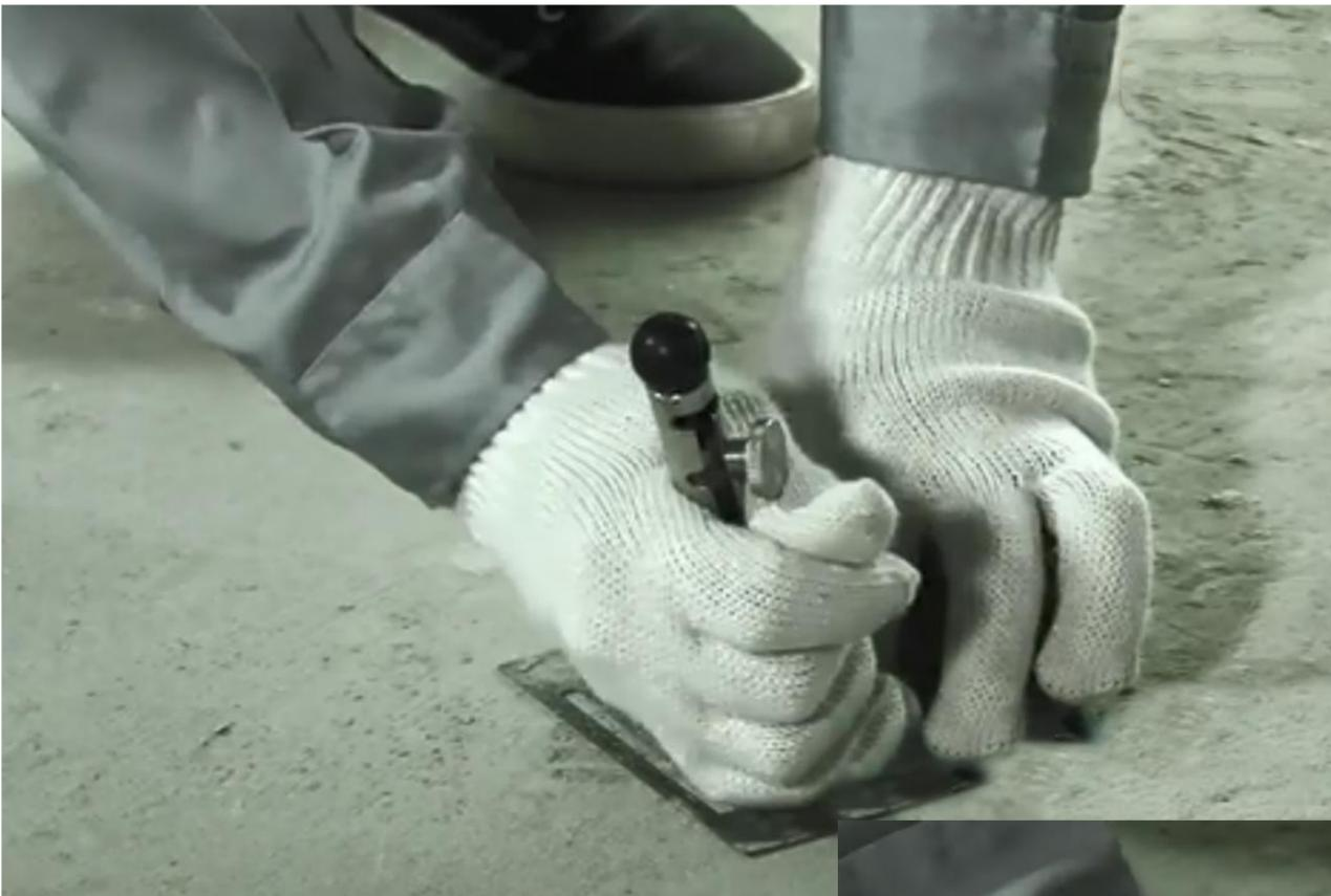
Using the hardness scratching tester to detect the hardness of ground surface.
